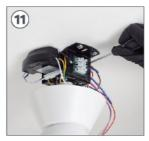
Connect the N wire from the driver with the neutral wire from your house wiring.
