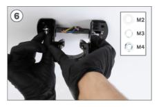
Insert pieces M2, M3 and subsequently the nut M4.
