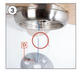
Connect the wires in piece  ${\bf D}$  to those of the fan joining the connections, each wire with the same colour.
