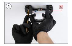
Mark on the ceiling with a pencil the 2 central holes of piece **K**, using the same piece as a guide.
