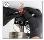
Once connected, place piece **O** screwing it in until it is secure.
