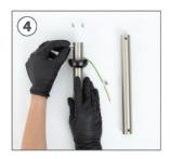
Remove the pin from the tilt support.
