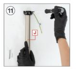
Tighten the two screws on the tilt support with the screwdriver.
