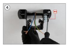
Using the screwdriver, tighten the screw **M2**.
