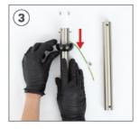
Using a screwdriver, remove the two screws from the tilt support of bar I.
