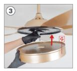
Pass the motor wires through the center hole of piece **G**.
