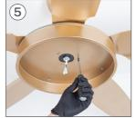
Firmly tighten the screws removed in step 1 so that piece G is properly attached.
