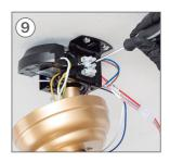
Connect the L wire from the driver with the LINE wire from your house wiring.
