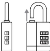
With the correct combination selected on the side, pull the lock shackle upwards to open the padlock.
