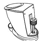
**EN** Remove the water tank from the coffee maker and put the injector into the water inlet hole. Then turn on the machine and press the steam button.
