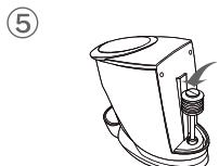
**EN** While the machine is running, press down on the injector until you see water coming out of the steam wand. If necessary, refill the injector.
