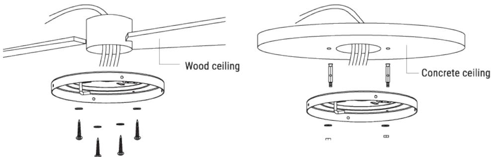
Please, drill an 8 mm in diameter hole on the concrete ceiling, and insert the bolt. Then, align the bracket with the hole and tighten with a nut.
