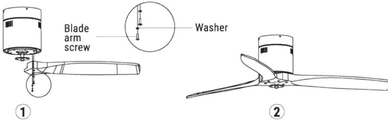
**Tip:** Washers for blade screws can be set on each blade screw prior to installing blades. Align the blade holes with the motor screw holes. Tighten all the screws once all the blades are attached. Before securing screws permanently, repeat with remaining blade arms.
