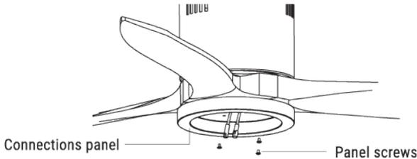
Attach the connections plate up to the bottom of the fan by inserting the set screw heads into the key hole slots. Rotate them to place and tighten them to secure the plate.
