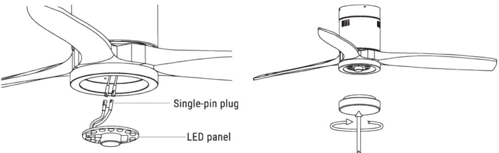
Connect the single-pin plugs of the connections plate with the ones on the LED panel. The LED panel is magnetized so it will be attached to the connections panel just by placing them together.
