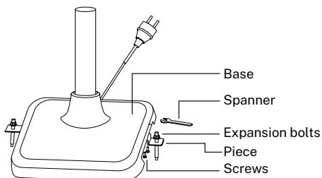
6. Fix the 2 pieces on the base of the product with the 4 M6x10 mm screws.
