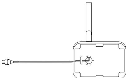
5. Pull the power cord gently out of the base as far as it will go. Secure the power cable under the base with the 2 supplied M4x12 mm screws.
