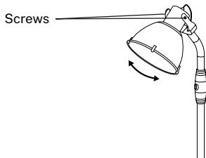
4. Rotate the head of the heater to the angle you need, then lock it with the 2 M4x12mm screws.
