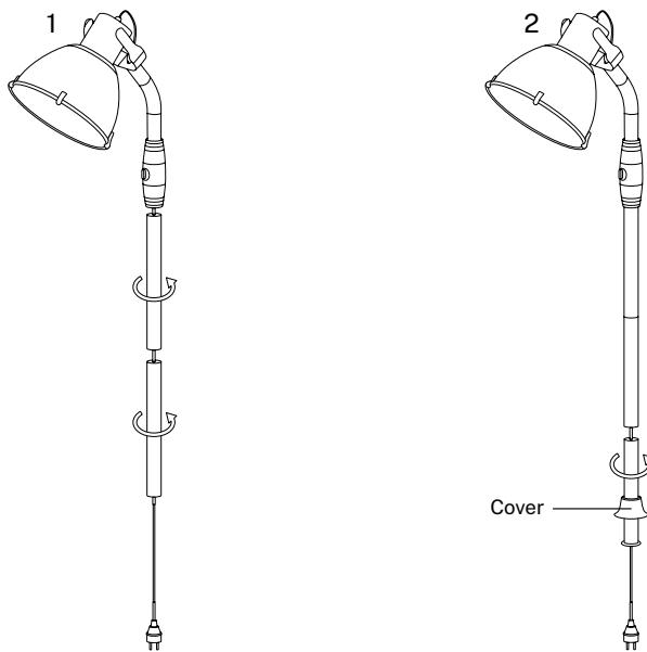
1. Connect the central tube parts to the central body of the product by screwing them together.
